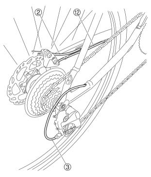
Check that the rear brake wire ②, rear shift wire ③, and speed sensor lead ⑫ are routed as shown in the illustration.
