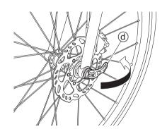
Move the lever (d) of the front axle (2) to "OPEN" facing the notch (e).
