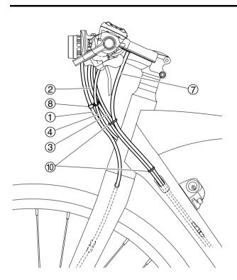
Check that the front brake wire ①, rear brake wire ②, rear shift wire ③, front shift wire ④, display unit lead ⑦, wire clip ⑧, and plastic locking ties ⑩ are placed as shown in the illustration.
