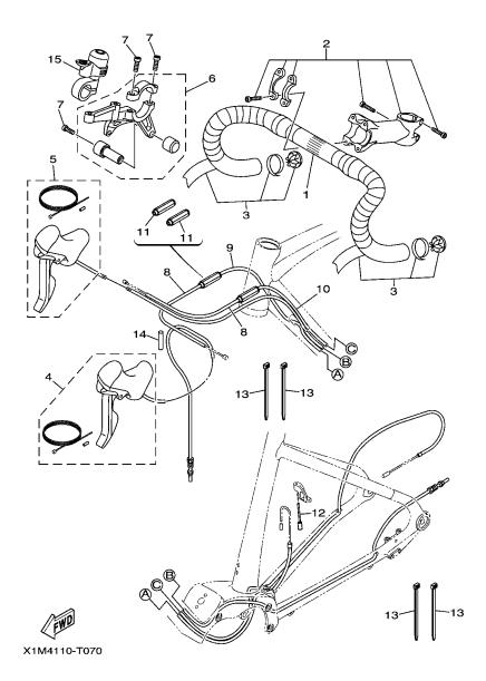
FIG. 7 STEERING HANDLE & CABLE
