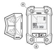
D. The hours value increases when the "▲" assist mode switch (f) is pressed while the "Hour" section of the clock (e) is flashing.
