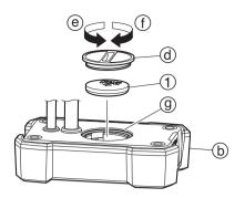
Turn the button cell battery cover (d) on the back of the display unit (b) in direction (e), remove it, then install the button cell battery (1).
