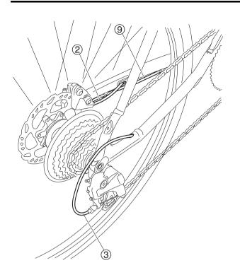
Check that the rear brake hose ②, rear shift wire ③ and speed sensor lead ⑨ are routed as shown in the illustration.
