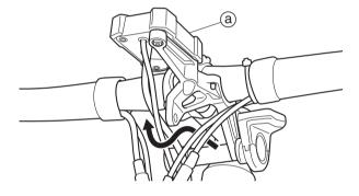
As shown in the illustration, install the bracket part of the display unit (a) to the side of the handlebar holder (b) and tighten the bolts (c) to the specified torque.
