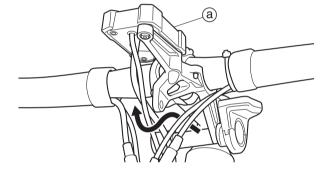
As shown in the illustration, install the bracket part of the display unit (a) to the side of the handlebar holder (b) and tighten the bolts (c) to the specified torque.
