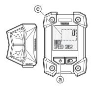
D. The hours value increases when the "▲" assist mode switch (f) is pressed while the "Hour" section of the clock (a) is flashing.
