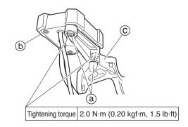
3. Installing the handlebar
