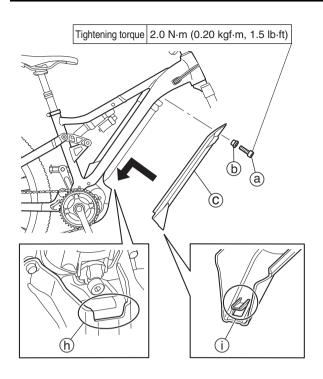
Hook the claw (i) of the battery cover to the hook part (h) of the motor cover, and then install the battery cover © along the frame.
