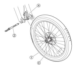
Move the lever a of the front axle 2 to "OPEN" facing the notch e.
