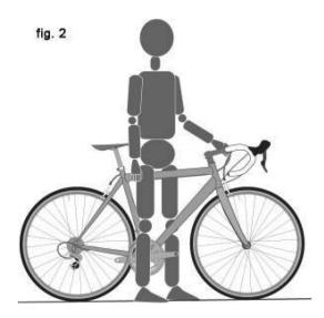
unpaved surfaces should give you a minimum of three inches (7.5 cm) of standover height clearance. And a bike that you'll use off road should give you four inches (10 cm) or more of clearance.
