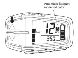
The Automatic Support mode, which enables automatic change to the optimal assist mode according to the riding conditions, can also be used.
