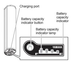
The battery pack equipped for the Yamaha e-Bike Systems is a lithium-ion battery. The lithium-ion battery is lightweight and offers superior capacity. However, it does have the following characteristics.
