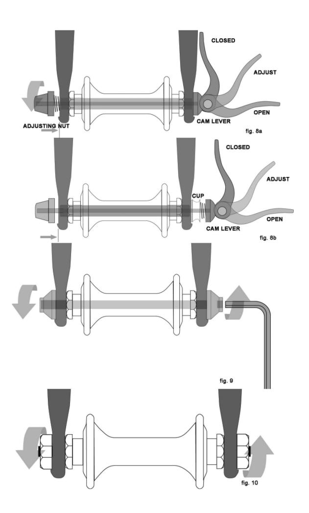
It is very important that you understand the type of wheel securing method on your bicycle, that you know how to secure the wheels correctly, and that you know how to apply the correct clamping force that safely secures the wheel. Ask your dealer to instruct you in correct wheel removal and installation, and ask him to give you any available manufacturer's instructions.
