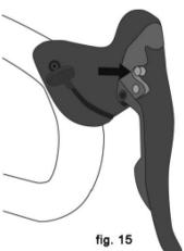
removed or reinstalled. When the brake quick release is in the open position, the brakes are inoperative. Ask your dealer to make sure that you understand the way the brake quick release works on your bike (see fig. 12, 13, 14 & 15) and check each time to make sure both brakes work correctly before you get on the bike.
